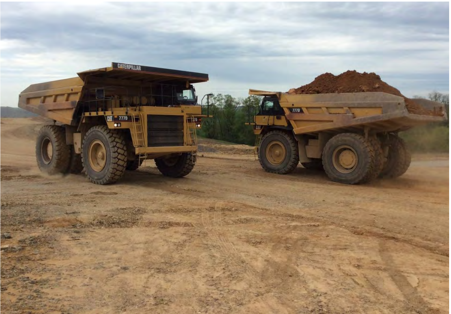
100-ton haul trucks used for earthmoving operations. These trucks were typically loaded by an excavator with a 10-cubic-yard bucket.
